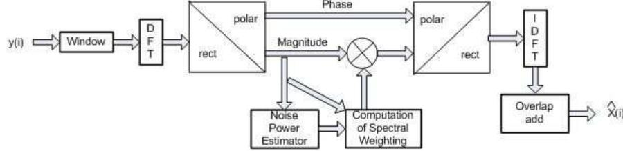
**Fig. 1.** Diagram of the Basic SS Method Used
